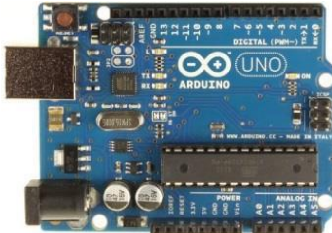
Figure 1 Arduino UNO R3 board with ATmega328P
